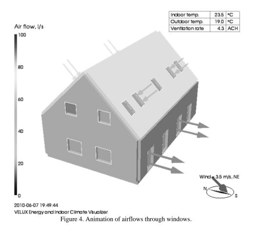
The animation is used to explore how the combination of ventilation controls and natural driving forces determine the magnitude and distribution of the airflows. It can be used to investigate stack effect, cross and single sided ventilation under different weather conditions during a year.
